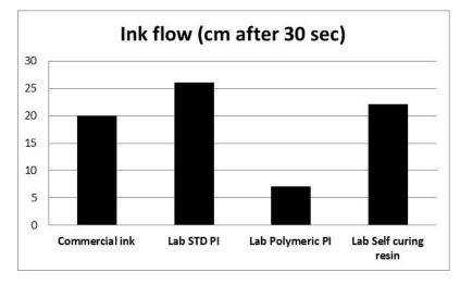
Fig.4: Ink flow in cm of black flexo inks, using 3 g of ink and 30° flow plate angle.
