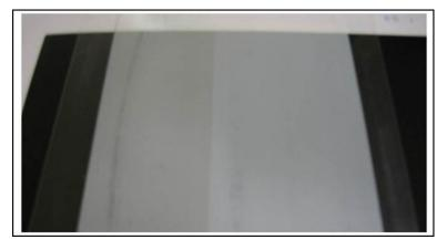
**Fig. 7:** Comparison of whiteness/yellowing: commercial white flexo ink (left) versus self-curing acrylate resin based white flexo ink (right) at 2 g/m<sup>2</sup>.
