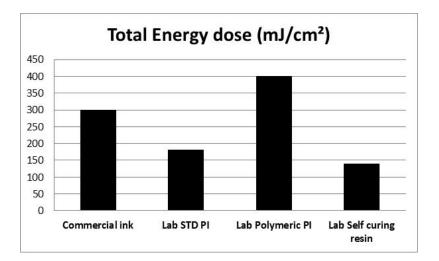
Fig.3: Reactivity of black flexo inks: total energy dose in mJ/cm<sup>2</sup> to obtain a dry film (1.2 g/m<sup>2</sup>).
