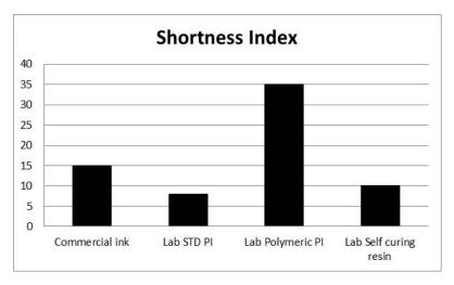
**Fig. 9:** Ink flow properties: shortness index (SI) of magenta offset inks. SI = ratio low shear viscosity/high shear viscosity.
