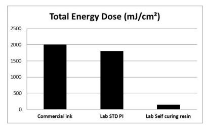
Fig.6: Reactivity of white flexo inks: Total energy dose in mJ/cm<sup>2</sup> to obtain a dry film.
