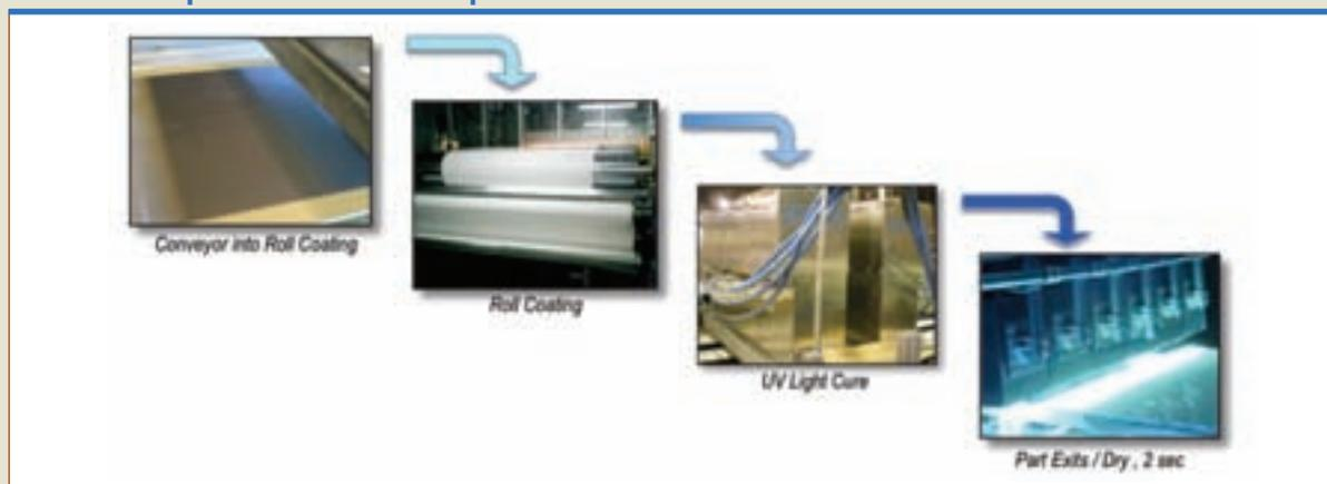
length—a very small overall footprint. The energy efficiency of the UV-cure system provided significant cost savings for the customer's operations, while the immediate quality inspection of the coated parts offered significant quality cost savings. The customer was also pleased to remove all solvents and VOCs from their coating operation, which offered a healthier and safer workplace for their employees.
