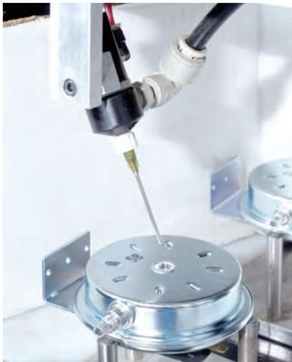
*Calibration screws on low-pressure air switches are covered with UV-cure adhesive to keep them in position and discourage tampering. Switching to a new adhesive and an automated dispensing/curing process has cut process time from five minutes to five seconds.*
