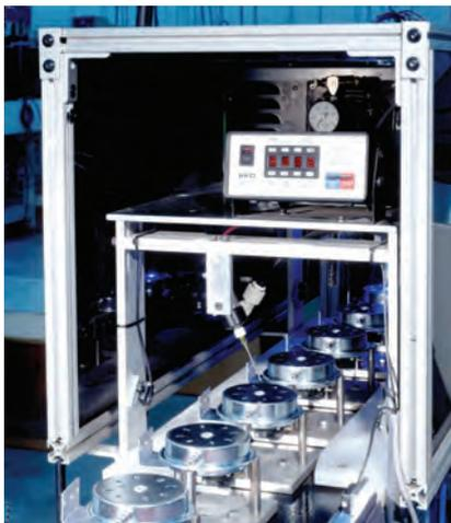
*New dispensing/curing lines have helped this pressure switch manufacturer eliminate bottlenecks and increase productivity more than 25%. Universal fixturing, dedicated dispense valve controllers and adjustable curing equipment give them the flexibility to handle any product configuration with just a few minutes of setup time.*
