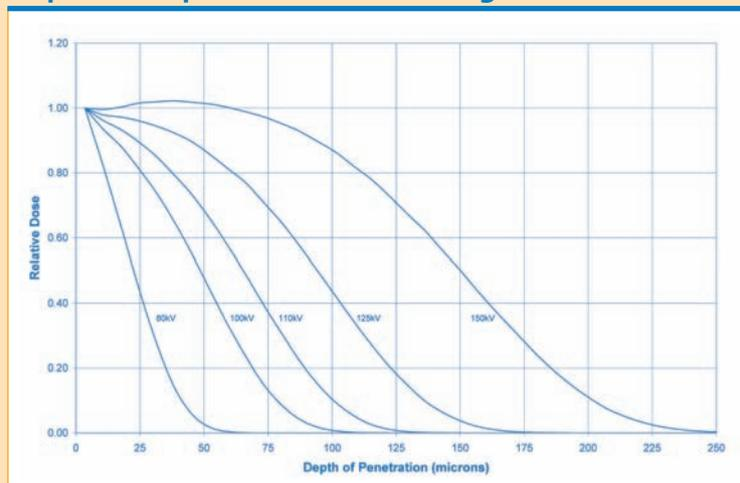
EB penetration is controlled by the accelerating potential (voltage) of the EB equipment. Figure 2 shows EB penetration as a function of voltage. Low-voltage EB equipment operating from about 70 to 125 kV is ideal for curing thin inks, coatings and film layers used in most printing and packaging applications.<sup>6</sup>
