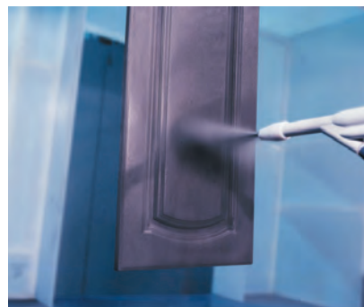
Powder coating being applied in a spray booth, which provides uniform airflow controlling the thickness of the applied powder.
