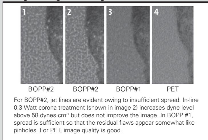
For BOPP#2, jet lines are evident owing to insufficient spread. In-line 0.3 Watt corona treatment (shown in image 2) increases dyne level above 58 dynes-cm<sup>-1</sup> but does not improve the image. In BOPP #1, spread is sufficient so that the residual flaws appear somewhat like pinholes. For PET, image quality is good.
