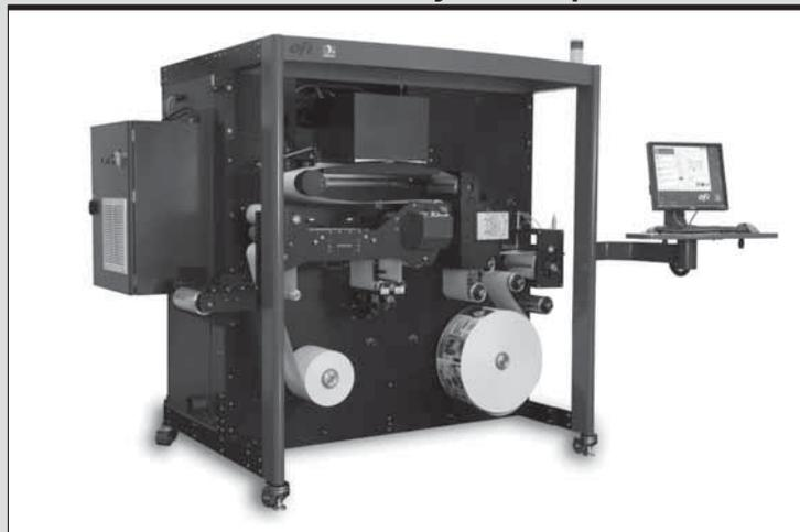
advantages of UV-curable inks is that it separates the ink solidification process after printing from the potential for drying in the nozzles. This enables quick curing after printing but enables good reliability of the print head.
