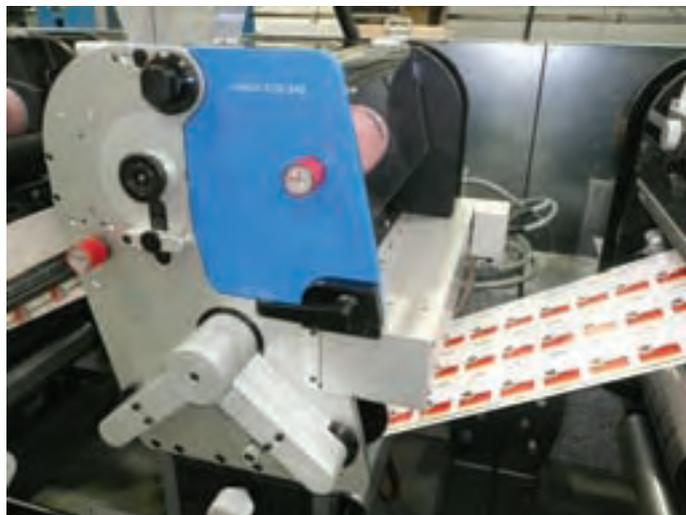
small size and easy integration of LED-based lamps compared to traditional mercury-based systems. Due to cost constraints, TIJ-based inkjet systems require small, affordable air cooled UV-LED systems that offer acceptable cure rates on a variety of print media.
