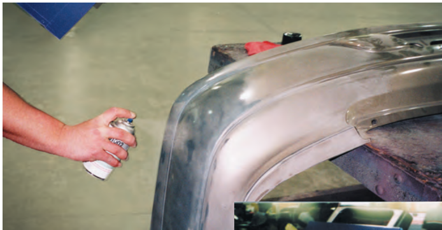
The UV-cured primer is sprayed to cover the damaged area.
