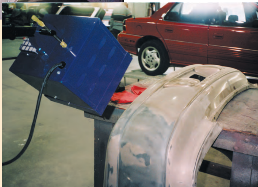
A low-energy lamp is used to cure the primer.
