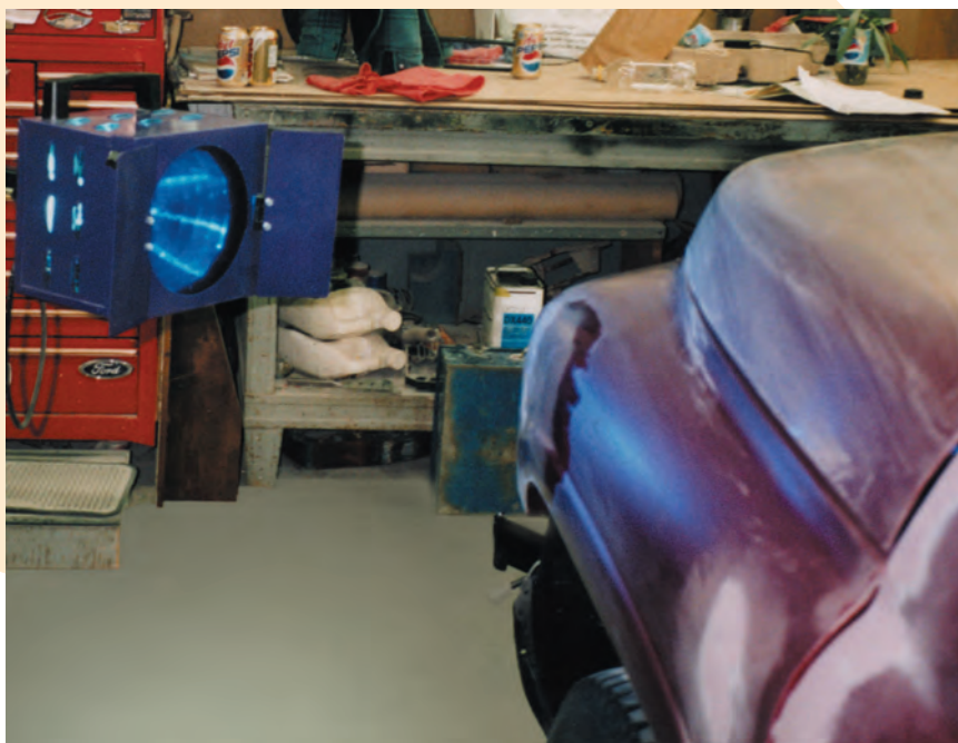
A UV-cured primer system makes the most of shop space since the UV primer can be applied and cured with a UV lamp anywhere in the shop.
