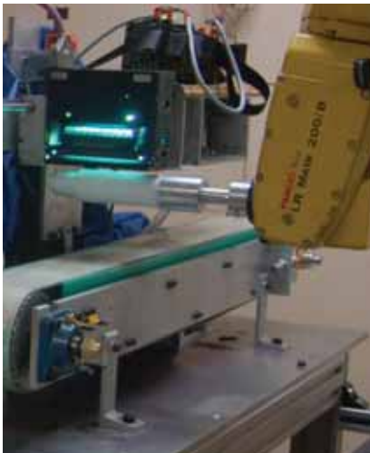
The way “around” line-of-sight limitations of UV is, quite literally, to move the parts so all surfaces are exposed.
