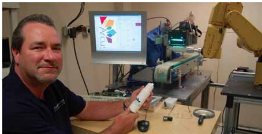
Three-dimensional shapes such as this shampoo bottle are easily decorated with robotic manipulation of the part under the print head and UV source.
