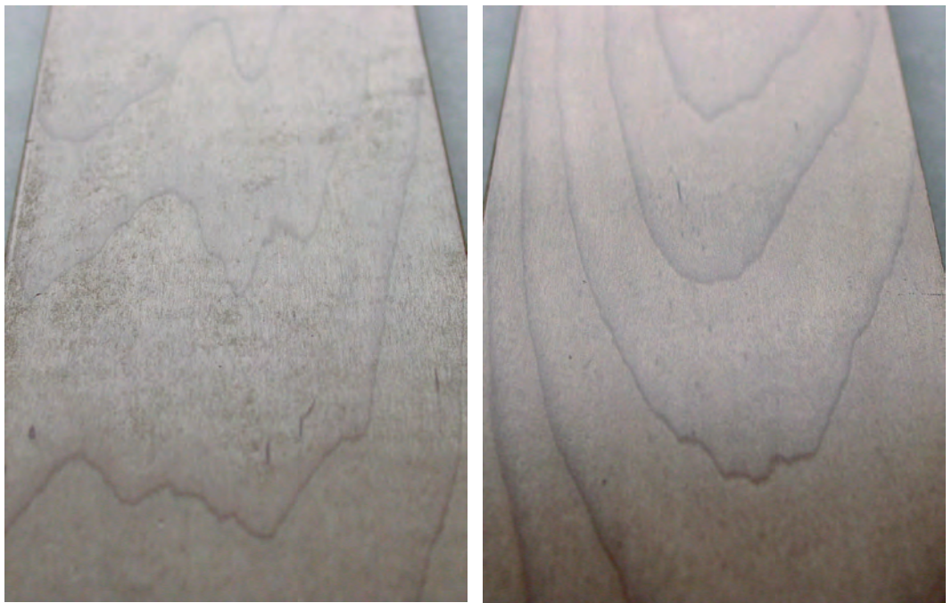
The proper seal coat application is illustrated in the picture on the left. Roll coat application of 100% UV curable was performed to achieve the surface appearance where dry spots and lack of build is observed. This application thickness enables ease of sanding denib and permits excellent finish uniformity upon topcoat application as shown on the right.
