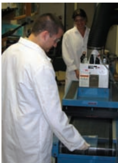
Timothy Morales and Elda Rueda making the first UV-polymer film using the new continuous photon output electrodeless lamp from Fusion UV Systems, Inc.
