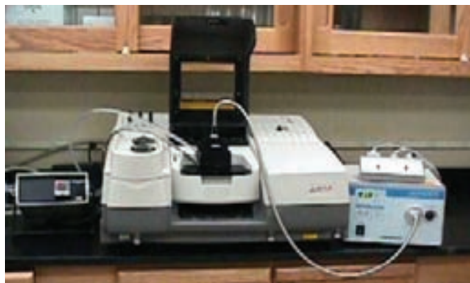
A fiber optic source is used to provide continuous or pulsed irradiation of a sample on a diamond crystal of IR spectrometer (attenuated total reflection sampling technique).
