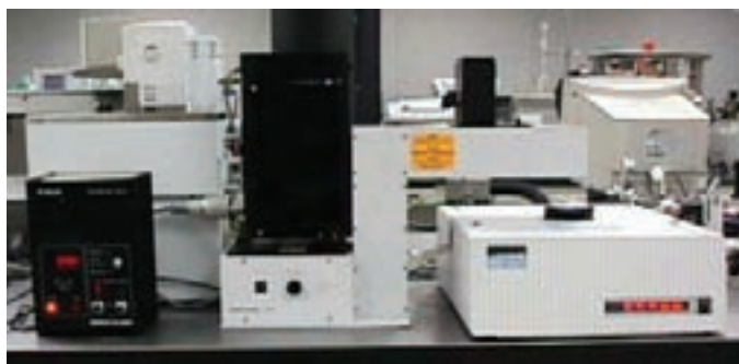
Lamp and power source are on the left. Sample and reference pans are irradiated simultaneously through quartz windows on the sample compartment at the top of the DSC unit.
