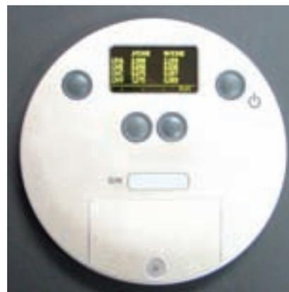
*Example of a radiometer that displays irradiance and energy density.*
