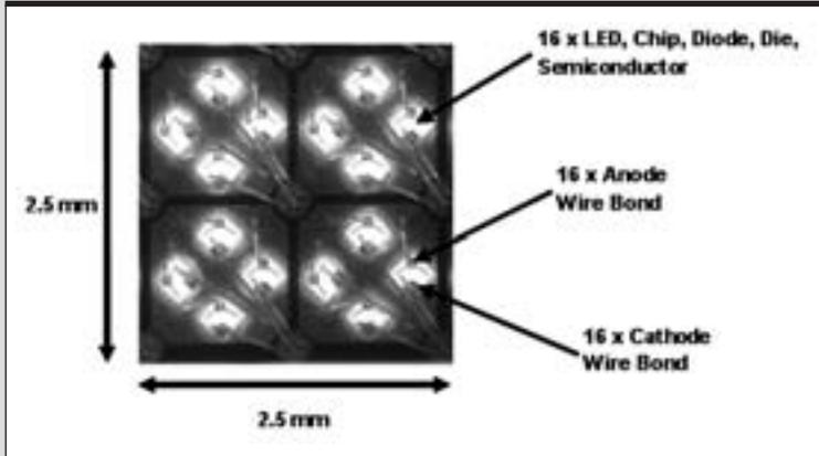
welding or thermal compression is used to electrically connect LED chips to a printed circuit board (PCB). One wire bond is made at the chip's positive terminal or anode while the other is made at the negative connection or cathode.
