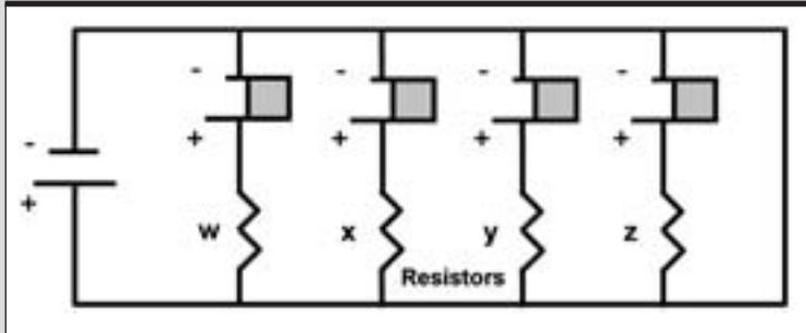
advantage of continued operation of all functioning LEDs even if one or more LEDs fail. In either type of circuit, it is important that the anode and cathode connections be alternated. This is because LEDs have polarity and current will only flow in one direction. Placing two anodes or two cathodes in sequence will disable the circuit.
