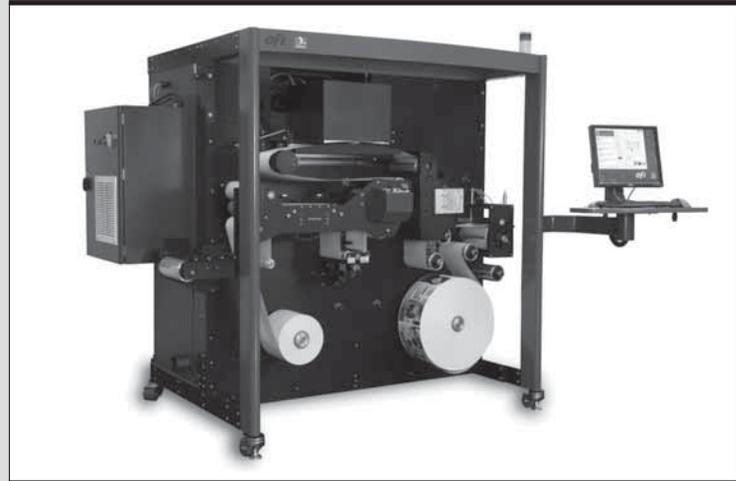
advantages of UV-curable inks is that it separates the ink solidification process after printing from the potential for drying in the nozzles. This enables quick curing after printing but enables good reliability of the print head.
