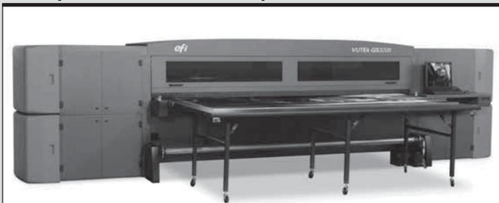
The print heads and lamps are mounted on a carriage that shuttles back and forth over the substrate. The printer can operate in various modes—laying down drops at a resolution that depends on the number of passes.
