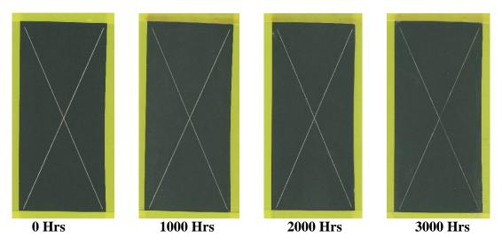
Figure 5. Corrosion Protection Of 2024-T3 Aluminum Alloy In ASTM B-117 Salt Fog Testing
