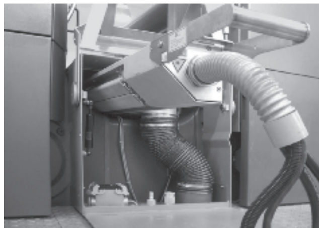
Gear-side view of interstation UV-curing unit from below.
