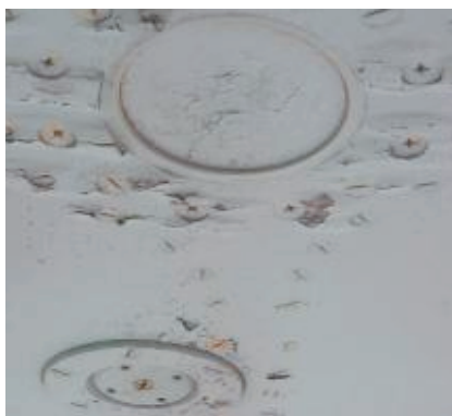
Typical aircraft corrosion often found near seams and fasteners.
