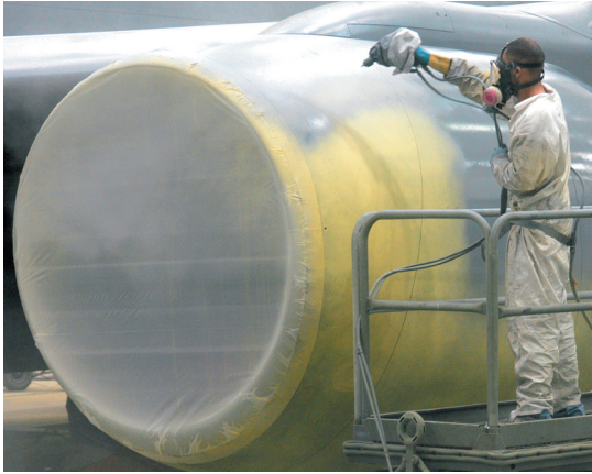
Application of a topcoat to a KC-135 Stratotanker engine nacelle at Oklahoma City ALC, Tinker AFB.
