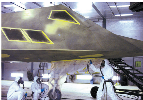
Application of a topcoat to an F-117A Nighthawk.
