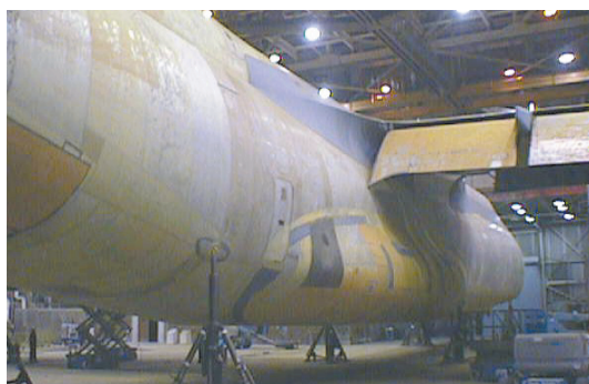
A stripped C-5 Galaxy waiting to be fully repainted. It is extremely difficult to completely remove all of the existing coating and prepare the substrate to a pristine condition prior to repainting.
