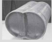
dimensional stability (e.g., with thin radiation reflector bodies or non-symmetrical thicker structures) is possible because of the lower internal stresses of a part cured at ambient temperature via EB. The ability to use lower cost tooling, even cheap tooling such as Styrofoam for internal mandrels allow for a form of the "lost wax process."
