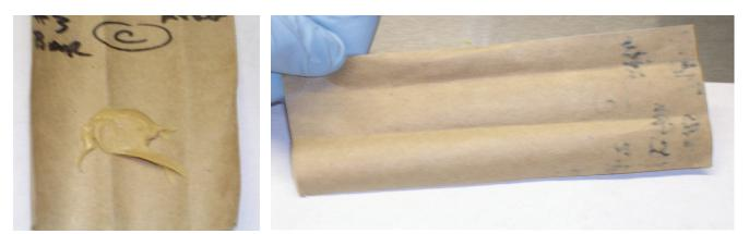
Peanut butter on kraft paper (left) and the reverse side showing no oil penetration (right).
