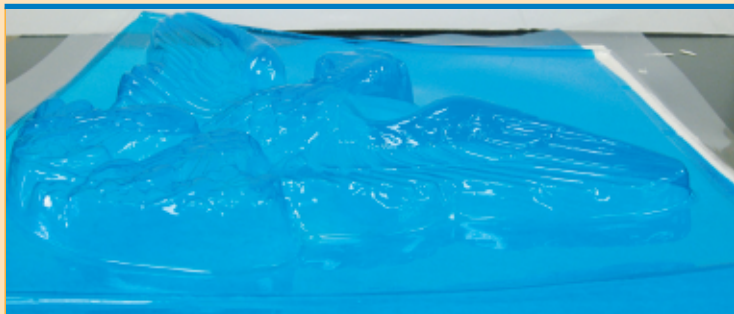
Drawn down on a flat sheet of PVC, then thermoformed
