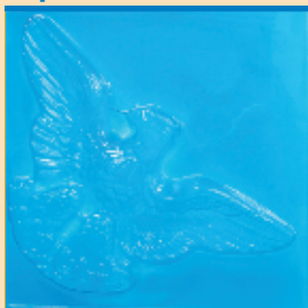
Drawn down on a flat sheet of PVC, then thermoformed
