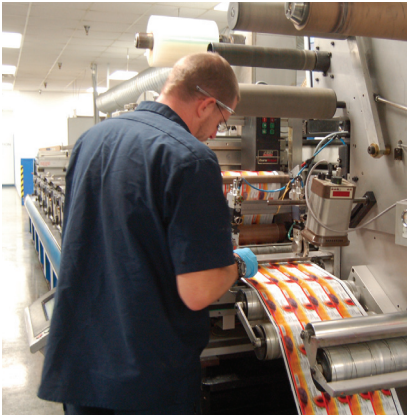
An operator inspects print quality at the end of a multistage UV-curing press equipped with UV lamps.
