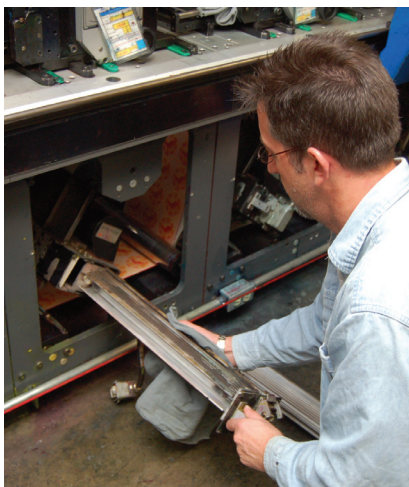
Changing an Ultrapack® UV module is as quick and simple as changing a toner cartridge on a printer.
