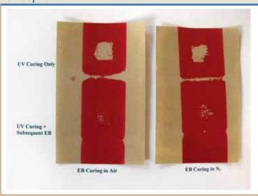
additional benefit of the dual UV/EB curing is the elimination of the need to inert the EB-curing process. These systems appear to offer good potential for commercial package printing installations.
