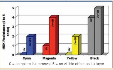
exposure. However, tape adhesion remains poor in all cases. The poor tape adhesion is likely due to limited UV energy reaching the ink/substrate interface with this high-density (2.69) ink layer. After EB exposure, MEK resistance is greatly improved and appears to be about the same for all
