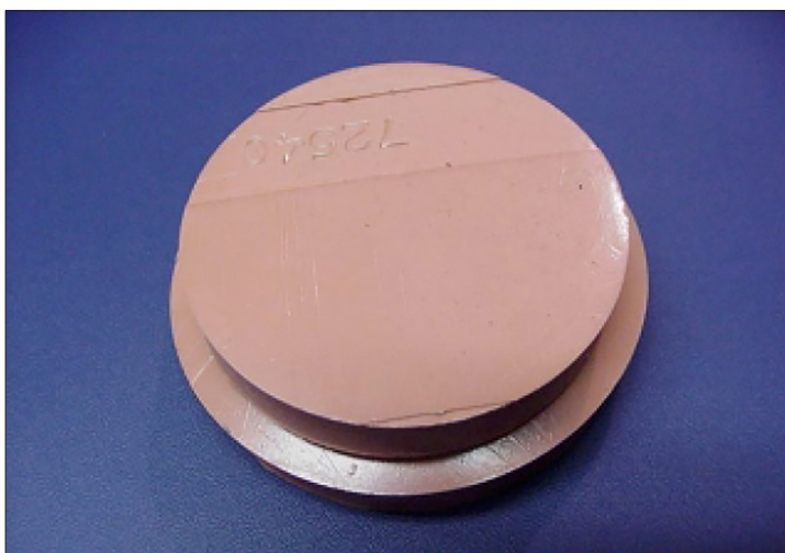
PHOTO 2. EPDM sample immersed in conventional ink for seven days. Lower button is test sample. Upper button is an original-size control sample for comparison.
