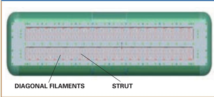
from the filament and create a cloud around them. These electrons are then extracted and accelerated by applying a series of positive grid voltages. The tungsten filaments are spaced every 76 mm across the entire width of the electron accelerator. So, for example, a 1,370 mm-wide EB processor would have 20 filaments about 200 mm long placed parallel to each other.
