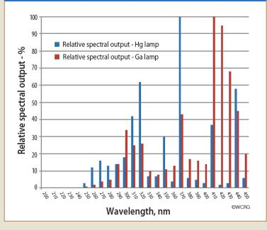
Relative spectral output of Mercury- and Gallium-doped lamps
