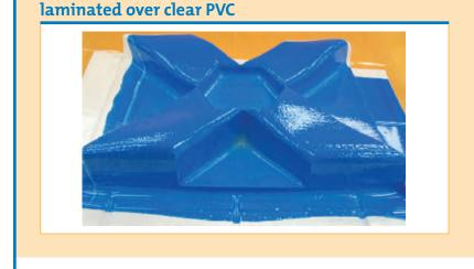
Thermoformed cured ink drawn down over vinyl,
