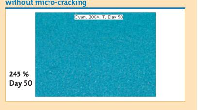
Micrograph of an elongated ink aged over a month without micro-cracking
