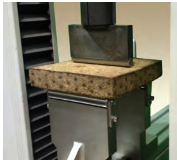
Mechanical testing fixtures used for testing mycological composites to provide (a) modulus of elasticity, modulus of rupture, and (b) screw withdraw strength following ASTM D1037.
