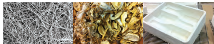
(Left) 140x magnification of mycelium; (Middle) agricultural waste from the cotton industry; (Right) grown biomaterial that serves as protective packaging, the mycelium is white.
