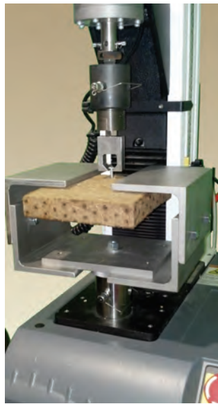
Mechanical testing fixtures used for testing mycological composites to provide (a) modulus of elasticity, modulus of rupture, and (b) screw withdraw strength following ASTM D1037.
