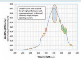
LEDs can be made at any wavelength along the curve, and the colored markers are positioned at commercially important wavelengths where relative size of the marker suggests market size for LEDs at those wavelengths. If UV-LED efficiencies improve to the levels of today's 450nm LEDs, they would be more than twice as efficient as mercury lamps and offer a wider range of UV wavelengths.
