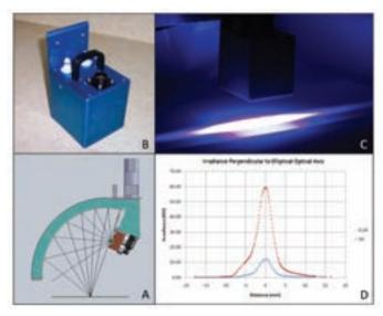
The operating concept is shown in (A) and a finished module in (B), actual operation in (C) and an intensity profile measured 80 mm from the base of the unit in (D). Operation is based on a proprietary LED and optical design intended to emulate the power levels and emission patterns of highpower, mercury-arc lamp systems.
