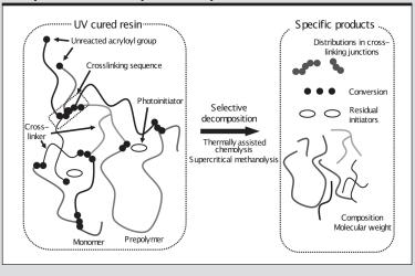
decomposition of the UV-cured acrylic resin. From the obtained fragments, some valuable information for conversion, residual initiator, composition and molecular weight of original monomer/prepolymer, and distribution in crosslinking junctions can be obtained.
