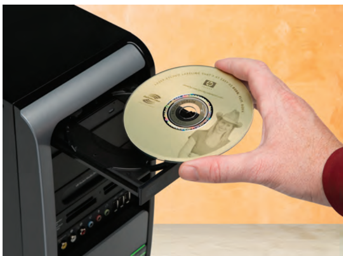
This UV-curable system consists of a LightScribe enabled drive, imaging software and the UV-cured coated media.
