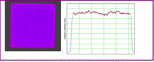
**Figure 5.** Illumination pattern (8 inch by 8 inch) produced SSD light source shows uniformity variation less than 4% at curing intensities.
