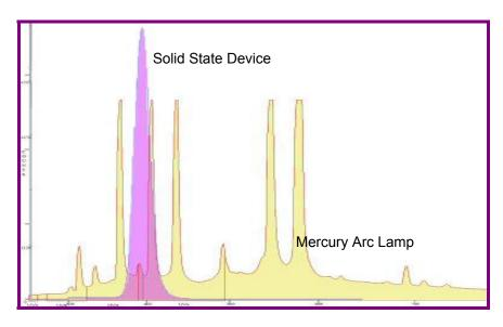
**Figure 6.** Spectral output of a medium-pressure mercury arc lamp and SSD, showing the SSD to be both more intense and have a more narrow band of emission.
