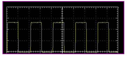
**Figure 8.** SSD sources can provide instantaneous pulses with <1 msec rise times, allowing variable intensities, on/off control, and programmable cure recipes in addition to traditional continuous cures.
