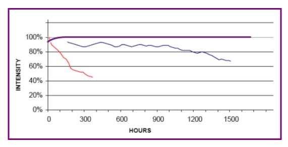
**Figure 4**. Lifetime data for two commercially available arc lamps and SSD Light Source. While no appreciable degradation was observed during this test, > 10,000 hrs is estimated for the SSD.
