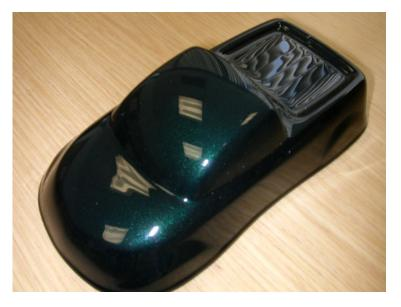
Figure 8. Photograph of a 3-D Form with a Basecoat/Dual Cure Clearcoat Finish.
