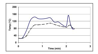
Figure 2 - Heating / curing profile applied on MDF (Solid line = surface temperature) (Broken line = temperature beneath the surface)
