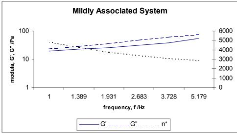
This example shows a mildly associated system that exhibits weaker structure than a strong associated system. G" is slightly dominant over G' indicating a potential for instability. Notice the mild dependency of the G' and G" moduli to frequency. Also, the complex viscosity exhibits a low dependency on frequency. Tan  $\delta$  = 1.4 (>1, <3). Flocculation and or settling may occur in this system.
