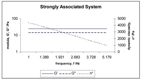
Note the relationship of each parameter to frequency. Both G' and G" show no dependency upon frequency and G' is dominant over the G" (more elastic than viscous) indicating a strong particle-particle association. The complex viscosity (n\*) exhibits rapid decline with increasing frequency. Tan  $\delta$  = 0.6 (<1). This system is stable, not prone to flocculation or settling and is considered highly structured.
