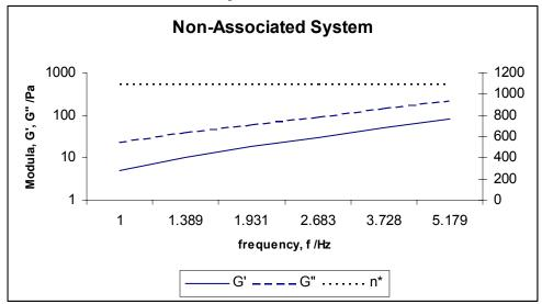
The relationships of G', G", and n\* to frequency in this system are opposite of that found in the strongly associated system. G" greatly dominates over G' with a high frequency dependence and the complex viscosity is totally independent of frequency. Tan  $\delta$  = 3.5 (>3). This system is unstable. It will likely undergo flocculation and settling. It exhibits poor structure and virtually no particle-particle association.
