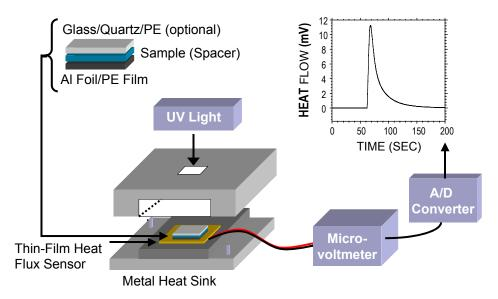
Figure 1. Diagram of the thin-film calorimeter (TFC)
