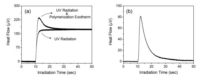
**Figure 5.** TFC exotherms of (a) the incident UV radiation and the polymerization of a 5 micrometer thick UV curable ink and (b) the polymerization exotherm after the heat from the UV radiation has been subtracted. Light intensity was 50 mW/cm<sup>2</sup>
