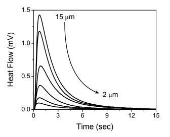
**Figure 4.** TFC polymerization exotherms of HDDA at various sample thicknesses. Samples contained 1wt% DMPA and were irradiated with light intensity of 50 mW/cm<sup>2</sup>.
