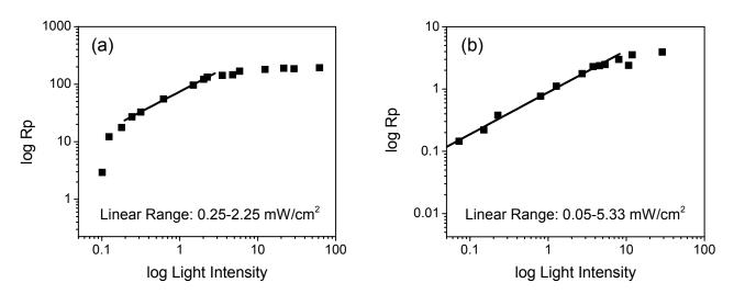
**Figure 3.** log-log plots of the polymerization rate (Rp) vs light intensity for 200 micron thick HDDA samples using the (a) photo-DSC and (b) TFC. All samples contain 1 wt% DMPA.
