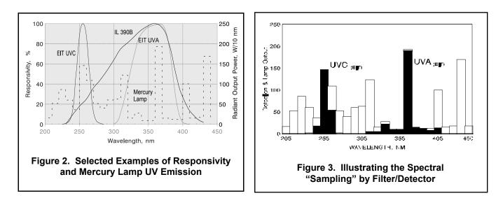
Spectral responsivity is the characteristic that differentiates wide-band radiometers from narrow-band radiometers. It can be easily seen, from Figure 2, that any of these yield very different measurements when exposed to the <u>same lamp</u>! Further, it should be noted that, at best, the data reported for any band is a *sampling* of the spectral power in that band. This is illustrated in Figure 3.
