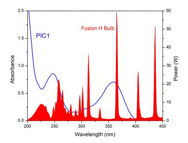
Figure 1. UV-Vis absorption spectrum of PIC1 and output spectrum of a medium pressure mercury lamp (Fusion H bulb).
