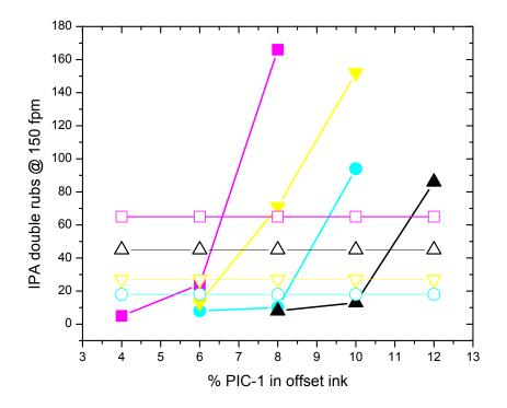
Figure 2. Isopropyl alcohol double rubs for ( $\Box$ ) standard process magenta, ( $\triangle$ ) standard process black, ( $\nabla$ ) standard process yellow, (O) standard process cyan, ( $\blacksquare$ ) magenta test ink, ( $\nabla$ ) yellow test ink, (●) cyan test ink and (▲) black test ink.
