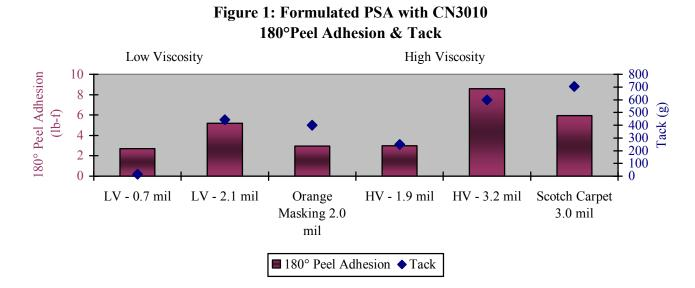
As with most PSAs, when the adhesive thickness is increased, the 180° Peel Adhesion, tack and SAFT are also increased. This is easily seen when comparing the two different application thicknesses for the two formulated UV cured PSAs.
