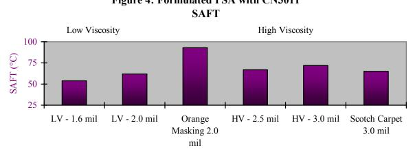
hieve a 2.5 mil adhesive thickness to achieve comparable results to the S **Figure 4: Formulated PSA with CN3011**
