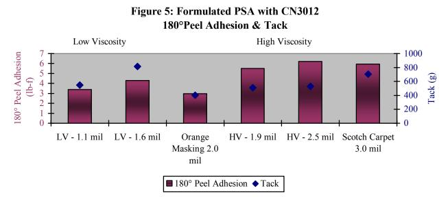
The low viscosity material seems to have a higher peel adhesion and tack than the commercial product being compared with (Orange Masking Tape). The higher viscosity formulated PSA is very strong even at lower adhesive thickness although it is being compared to the Scotch Carpet Tape (3.0 mil adhesive thickness).
