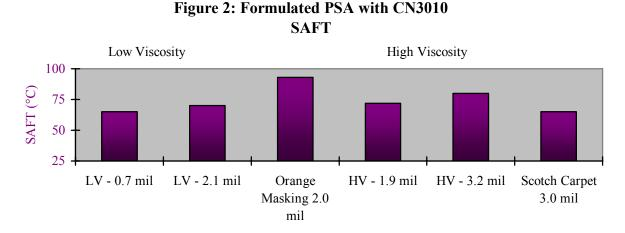
As shown in Figure 2, the adhesive thickness does play a role in the SAFT results. The Orange Masking Tape has a slightly higher SAFT than any of the formulated UV cured PSAs, but the Scotch Carpet Tape is lower than any of the experimental formulations.
