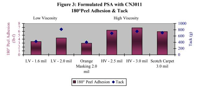
When looking at these formulated PSAs, the performance of the low viscosity #10 rod (1.6 mil adhesive thickness) UV cured PSA is similar to the Orange Masking Tape, but lower adhesive thickness to achieve similar results. A similar trend was seen with the high viscosity formulation, again using the #10 rod to achieve a 2.5 mil adhesive thickness to achieve comparable results to the Scotch Carpet Tape.
