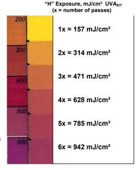
FIGURE 1 Visual Resolution vs Radiometer Measure of Exposure
