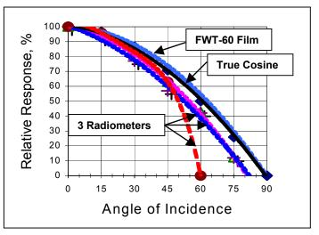
Figure 10 Cosine Function and Angular Response of Three Commercial Radiometers and FWT-60 Radiachromic Film
