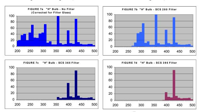
FIGURES 7a – 7d Relative Spectral Exposure with SCS<sup>(5)</sup> Series Cutoff Filters
