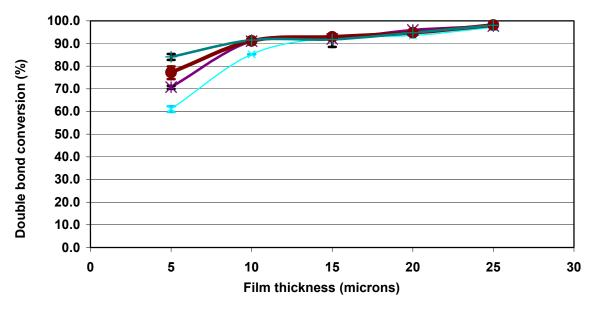
Fig. 9 Double bond conversion as a function of film thickness in a 25 microns and  $I_0$  (mW/cm<sup>2</sup>), EB8402/SR506 (3:7), Irg. 819 2.5% in air with the same total UV dose and at different cure speeds
