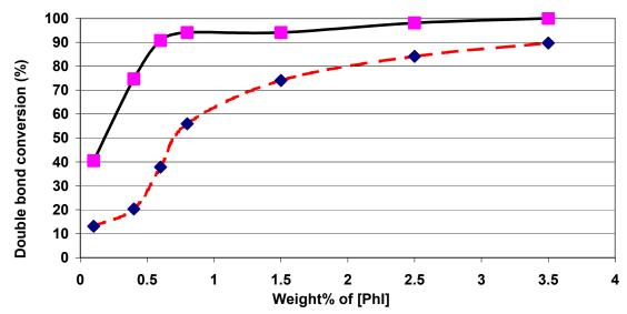
Fig. 5 Double bond conversion of top 5 microns and bottom 5 microns in a 25 micron film as a function of [PhI], 67 m/min, EB8402/SR506 (3:7), in air
