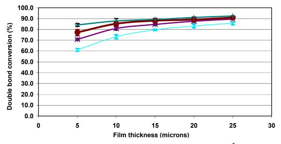
Fig. 7 Double bond conversion as a function of film thickness and  $I_0$ (mW/cm<sup>2</sup>), EB8402/SR506 (3:7), Irg. 819 2.5% in air with the same total UV dose and at different cure speeds
