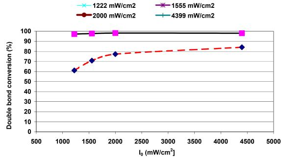
Fig. 8 Double bond conversion of top 5 and bottom 5 microns in a 25 micron film as a function of UV light intensity, with the same UV Dose and at different cure speeds, EB8402/SR506 (3:7) with 2.5% Irg. 819, in air
