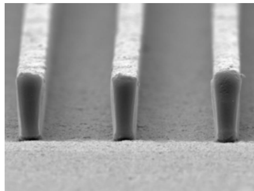
b. Pattern Feature: 10/26 μm line and space Exposure: Solid state UV direct imager (355 nm)
