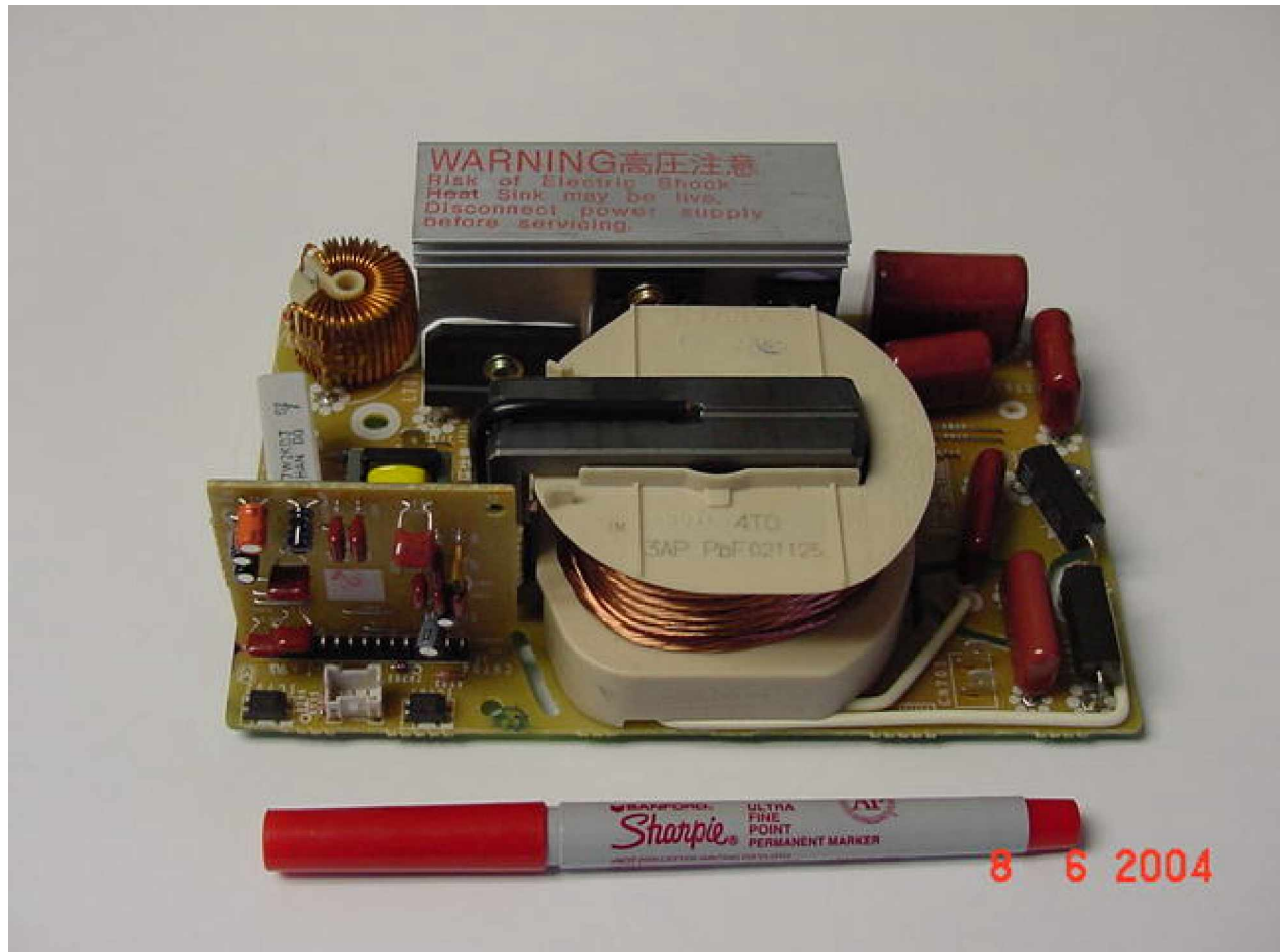
Fig. 6. 1.5 kW High Voltage Solid State Power Supply for running 1 kW magnetrons.
