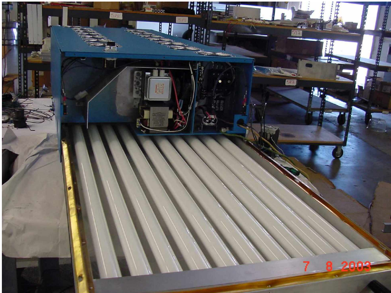
Fig. 5. Dual Magnetron 25"×43" Output UV Window Multi-Lamp UV System. Magnetron power Supply and Lamp Cartridge are shown.
