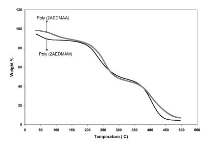
**Figure 3. TGA** of Poly[(2-acrylate)ethyl-dimethylammonium acrylate] and Poly[(2-acrylate)ethyl-dimethylammonium methacrylate], Poly(2AEDMAA) and Poly(2AEDMAM), respectively; at a heating rate of 10 °C/min.
