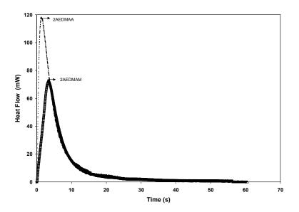
**Figure 1.** TFC polymerization exotherms of (2-acrylate)ethyl-dimethylammonium acrylate and methacrylate, 2AEDMAA and 2AEDMAM, respectively with a 25.5  $\mu$ m of thickness. Samples with 1 % of Irgacure 651 were irradiated with a light intensity of 32 mW/cm<sup>2</sup>.
