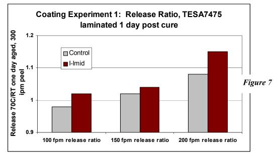
TESA7475 acrylic test tapes were affixed to each cured coating right after cure for RT and 70C laminate aging and peel release determination as described above. A post cure release ratio determination was carried out 2 weeks after coating and cure to mimic a typical inventory situation where release liner is shipped days or weeks after coating/curing of the release coating. 70C/RT aged release ratio results were recorded and are displayed in **Table 4**.
