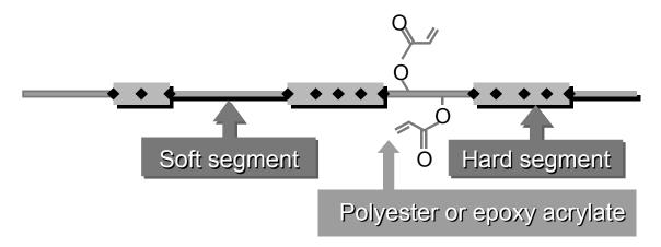
Coatings based on PUDs exhibit the highest growth potential in the wood market. The key property of this type of coating is its similarity to conventional PUR coatings – i.e. application methods, drying times and performance attributes.
