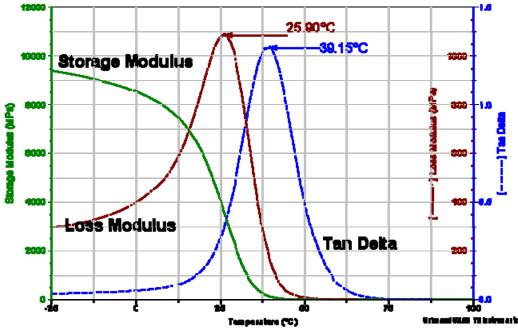
**Diagram 6.** DMA graph of CN2285 from -25° C to 100° C.
