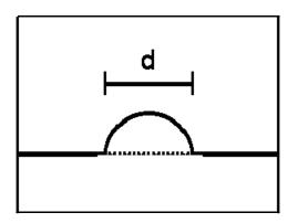
**Diagram 5.** Simple deformation using a dye with a semicircle end.
