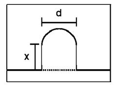
Diagram 6. Complex deformation with a draw and a semicircle end.
