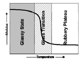
**Diagram 1.** Graphic representation of a thermoplastic system. The striped area represents the glass transition where the polymer changes from a glassy to a rubbery state.
