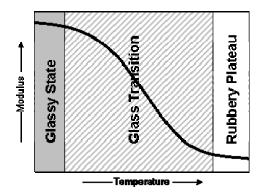
**Diagram 2.** Graphic representation of a thermoset system. The striped area represents the glass transition where the polymer changes from a glassy to a rubbery state.
