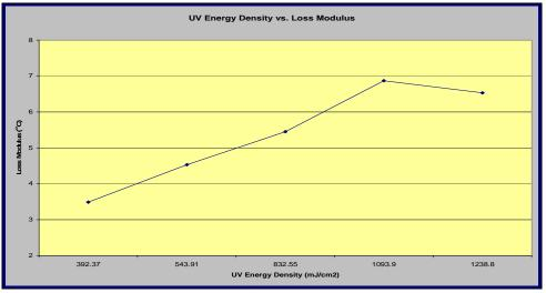
Figure 6 Loss Modulus & Transition (Tg) vs. UV-A Energy Density
