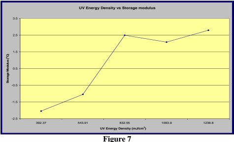
Storage Modulus  $\alpha$ -Transition vs. UV-A Energy Density
