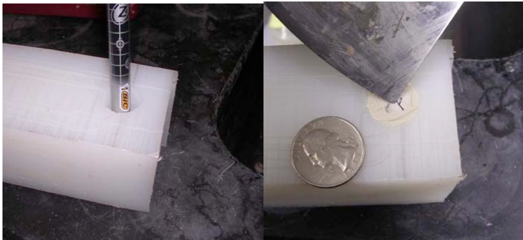
Figure 2. A hole was drilled in block of polyethylene. The resin, initiator and filler (calcium carbonate) were placed into the hole. The front was ignited with a lamp, and seconds a rock-hard material was formed.
