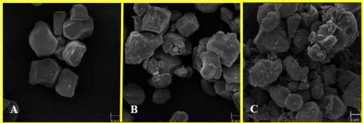
**Figure 3.** SEM micrographs of unmodified starch (A), simultaneously illuminated starch-g-PS (B), and 15-min pre-illuminated starch-g-PS (C).
