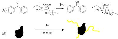
Figure 1. (A) Formation of radical on starch particle using benzophenone. (B) Formation of starch-gpolymer.
